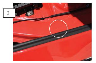
Thoroughly clean the upper frame rails with soap and water. Once completely dry, wipe the section of the frame rail with the stamped numbers with the supplied alcohol wipes. Once dry, apply the supplied adhesion promoter. Allow the promoter time to haze dry.
