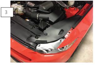
Test fit the part before removing the tape backing from the 3M Dual Lock. Do not install the clips at this time.
