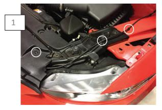
Begin by using a flat head screwdriver to carefully remove the outer radiator shroud push clip. Then carefully remove the (2) cable retaining clips on the hood latch cable. These will be left loose.
