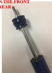
Use the provided o-rings on the REAR shocks below the bumpstops for lowered applications
