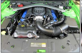
1. Disconnect The Negative Battery Terminal. Additional Installation Note: This Intake system can also be installed on a Mustang GT 5.0L with the Boss intake manifold conversion and contains the fitting required to connect the brake aspirator line for AT equipped vehicles.
