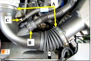
2. A) Loosen the hose clamps on the factory intake tube B) Squeeze the clamp and disconnect the resonator from the air intake tube. C) Carefully depress the hose lock tabs, and disconnect the crank case breather line and the brake aspirator line (if equipped, AT models only). **D**) Remove the factory intake tube.
