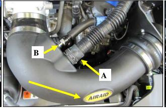
11. Install the Airaid Intake Tube into the couplers as 12. A) Install the Airaid Premium Filter onto the filter shown, and tighten all Hose Clamps. A) Reconnect the adapter and tighten the hose clamp. B) re install the Reso-Resonator tube to the Airaid Intake using the OEM nator tubing into the factory Stand off. clamp. B) Reconnect the breather line/lines to the Aluminum Fittings depending on your application. Apply the Airaid Decal onto the Tube as shown.
