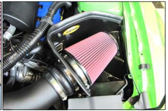
13. Reconnect the Mass Air Flow sensor, which is now 14. Install the Weather Strip onto the Cool Air Box with the contoured edge rolling away from the filter. Start at the front of the vehicle and work your way back.
