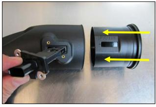
intake tube using two provided 8-32x3/8" screws (#12). **Do Not Use The Factory Screws!**
