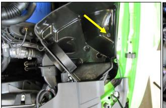
8. Install the Cool Air Box into the vehicle. Make sure that the Air inlet mates with the factory duct, and the two locating pins on the bottom align with the factory grommets. Next reinstall the factory bolt that was removed in step #3 through the steel sleeve and grommet and into
