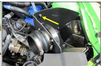
**9.** Install the hump hose onto the filter adapter using two #72 hose clamps (#13) as shown. Leave the two hose clamps loose for now. Transfer the Resonator stand off from the factory air box into the Cool Air Box.
