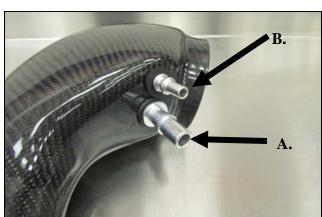
7. Install the Grommets and Fittings into the Airaid Intake 8. Install the filter adapter (#4) using three 1/4-20 button Tube (#2): A) All models will require the use of the 5/8" Fitting (#15) and the 5/8"Grommet (#12). **B)** Automatic transmission equipped vehicles will also use the 3/8" Fitting (#14) and 3/8" Grommet (#11). Manual transmission vehicles will not need the 3/8" components and will use the Blind Grommet(#13
