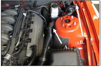
**4.** Remove the resonator assembly from the vehicle. A. Slide the hanger off of the strut tower tab
