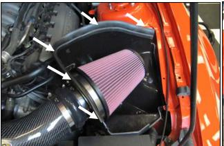
13. Install the Airaid Premium Filter (#1) onto the Flter Adapter and tighten the hose clamp. Install the Weather Strip (#7) onto the **CAB** with the contoured edge going away from the filter. Start at the front of the vehicle and work your way back.
