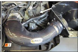
12. Install the Airaid Intake Tube into the couplers as
