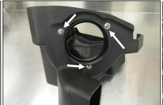
head bolts (#9), and Fat Washers (#8) into the Airaid Cool Air Box (CAB) (#3) as shown.
