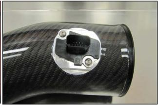
5. Insert the Fire Wall Plug (#16) into the resonator hole. 6. Using the supplied Torx bit, (#19) remove the MAF sensor from the factory airbox and transfer it into the Airaid Tube assembly (#2).
