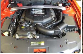
**Disconnect The Negative Battery Terminal!** 1. If so equipped, remove the strut tower brace, then remove the engine cover by simply lifting it up, and set
