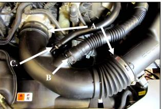
2. A) Loosen the hose clamps on the factory intake tube B) Squeeze the spring clamp and disconnect the resonator from the air intake tube. C) Carefully depress the hose lock tab, and disconnect the crank case breather line and the brake aspirator line if equipped, (AT models only). **D)** Remove the factory intake tube.
