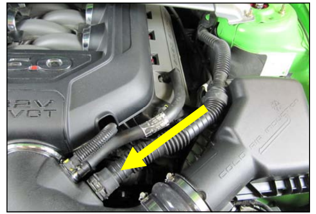
12. Resonator Delete Install Option: Airaid has made it possible to eliminate the factory induction resonator if you so desire. The removal of the resonator from the intake has no negative effect on the performance of this kit.
