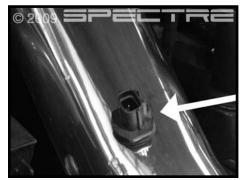
Step 13 Install IAT in the grommet installed in step 11. Be careful not to push the grommet through the hole.
