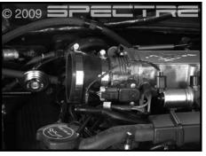
Step 8 Install the 3.5" - 3" coupler to the throttle body using the included clamp. Install a 3.5" hose clamp on the large side of the coupler, but do not tighten.
