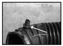
Step 12 Remove the IAT from the stock intake tube.
