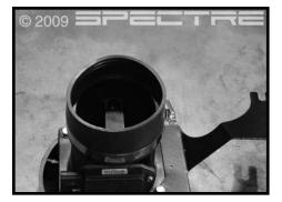
Step 7 Install the 3.5" coupler to the MAFS and secure with the included clamp. Install a second clamp, but do not tighten.
