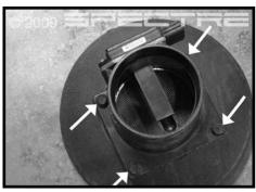
Step 5 Remove the 4 bolts retaining the MAFS to the air box assembly. Remove the MAFS. Carefully remove the screen assembly as it will not be reused.
