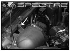
Step 4 Remove the 8mm bolt and remove the stock air filter box assembly.
