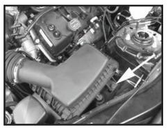
Step 4 Remove the factory air box and tube assembly by removing the 10mm bolt and lifting it out.
