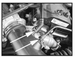
Step 2 Disconnect the 2 hoses from the factory air intake tube.
