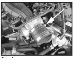
Step 8 Install the reducer coupler over the throttle body and secure with a supplied clamp. Install a second clamp but do not tighten at this time.
