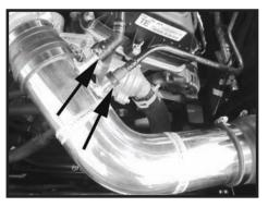
Step 11 Reconnect the factory vent lines to the intake tube.
