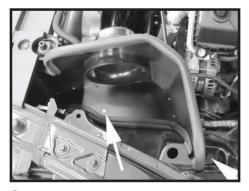
Step 7 Install the heat shield and secure it using the supplied hardware. Fully tighten all mounting hardware.
