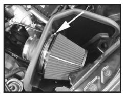
Step 9 Install the filter and securely fasten to the velocity stack adaptor.
