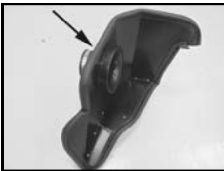
Step 10 Assemble the heat shield with the tabs placed on the outside of the heat shield (side with arrow). Place the velocity stack adapter in the heat shield and install the supplied reducer coupler making sure the coupler is pushed completely against the heat shield. Once the adapter and coupler are tight against the heat shield, tighten the clamp. Make sure that the clamp for the intake tube is installed but left loose at this time. Dress the heat shield with rubber seal as shown. This may require trimming to the correct length.
