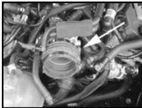
Step 13 Install the flex coupler over the throttle body and secure with a supplied clamp. Install a second clamp but do not tighten at this time.
