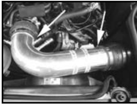
Step 16 Install the intake tube. Once in the desired location and everything fits in place, tighten the clamps.
