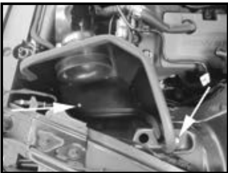
Step 12 Install the heat shield and secure it using the supplied hardware. Fully tighten all mounting hardware.
