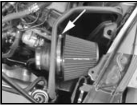
Step 15 Install the filter and securely fasten to the velocity stack adaptor.
