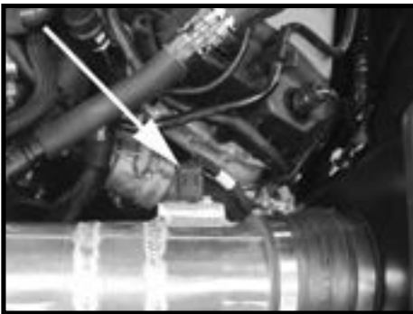
Step 18 Connect the wire extension harness into the MAFS harness on the vehicle then connect the harness to the MAFS connector by pushing the connector on the sensor. Once bottomed out push the red clip towards the tube to lock in place.
