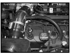
Step 17 Install the supplied 5/8" breather hose from the valve cover to the intake tube as shown.
