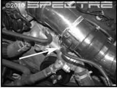
Step 16 Connect the MAF sensor harness. Push the red clip towards the tube to lock in place.
