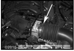
Step 4 Loosen the hose clamp at the throttle body.
