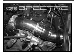
Step 15 Install intake tube that was pre assembled in step 11. Rotate tubes until everything is aligned properly and tighten the clamps.
