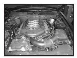
Step 2 Remove the engine cover by lifting on all the corners.
