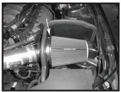
Step 20 Install the filter and securely fasten to the velocity stack adaptor.
