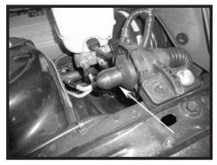
Step 19 Install the supplied cap over the valve that the roar tube was removed from in Step 4.
