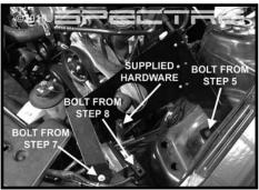
Step 11 Install the heat shield and secure it using the bolts removed in steps 7 & 8, and the supplied 8mm bolt, fender washer and lock nut as shown. Fully tighten all mounting hardware.
