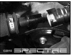
Step 2 Disconnect PCV tube from the intake by pushing on the green tab and pulling the tube off.
