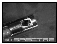
Step 13 Install factory MAF Sensor on the long intake tube using the supplied Phillips head screws.
