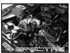
Step 14 Install 3" coupler with clamp onto throttle body. Fully tighten the clamp on the throttle body side.
