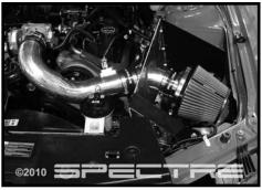
Step 18 Install the filter assembly onto the intake assembly. If necessary, adjust rotation of the short tube so that the filter is not touching anywhere on the car body. Once you have the filter positioned correctly, fully tighten all clamps.
