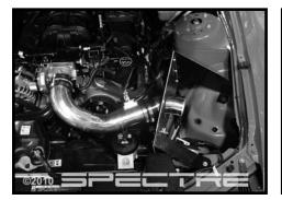
Step 16 Install the 3" coupler with two 3" hose clamps. With the coupler installed half way onto the tube, fully tighten the clamp which is over the tube. Insert the short Spectre intake tube through the grommet in the heat shield and into coupler. Ensure that MAF sensor calibration sleeve is fully seated, making contact with both tubes.
