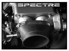
Step 14 Install the 5" hose clamp on the oval side of the coupler. Install the coupler onto the throttle body with the PCV tube pointing toward the passenger side. Fully tighten the clamp.
