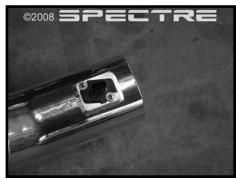
Step 16 Install the sensor in the new intake tube using the supplied Phillips head screws.
