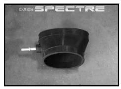
Step 13 Install the PCV fitting into the oval boot from the inside. **Ensure that it is completely** seated in the boot.
