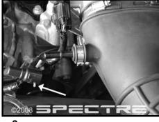
1- MAF sensor calibration insert
