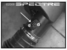
Step 15 Remove the mass air flow sensor from the stock intake tube.
