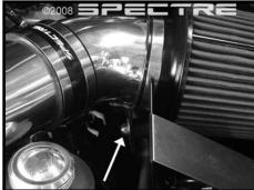
Step 22 Secure the intake to the rubber mount using a fender washer and lock nut.
