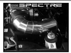
Step 17 Place a 4" hose clamp on the throttle body coupler and install the new intake tube as shown. Snug up, but do not fully tighten the hose clamp at this time.
