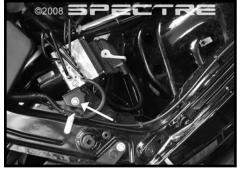
Step 6 Remove the bolt shown in the picture and set it aside for later use.
