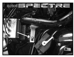
Step 10 Using the bolt removed in step 7, install the lower heat shield bracket as shown. Leave the bolt loose at this time.
