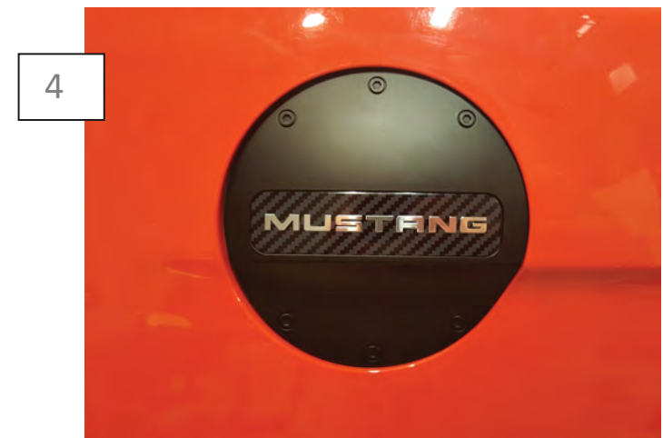
Slowly close fuel to ensure proper quarter panel clearance.
