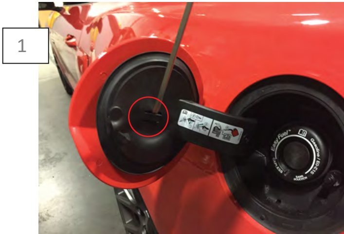
Open the factory fuel door. Using a small flat head screw driver, apply light pressure on the center clip.
