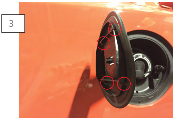
Line up the fuel door's (4) alignment tabs. Slide the fuel door onto the hinge until it clips.
