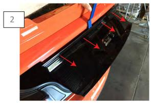
Use the panel removal tool to gently separate the factory deck lid panel from the deck lid.
