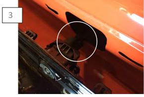
Unplug the reverse camera. Then remove the panel from the vehicle.
