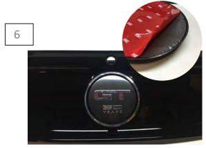
Test fit the emblem on the center of the decklid panel, then peel the 3M tape backing from the emblem. Center the emblem and apply firm even pressure to ensure proper adhesion to the decklid panel.
