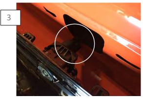
Unplug the reverse camera. Then remove the panel from the vehicle. \*\*Note Reverse Camera will be removed and reinstalled on to the MP Concepts panel.
