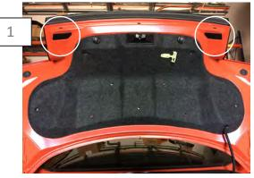
Using a panel removal tool, remove the caps covering the deck lid panel bolts. Then, remove the (4) 7mm screws.
