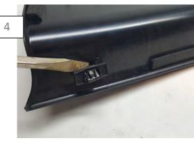
Remove the factory (4) push clips across the top of the decklid panel. Transfer the clips to the MP Concepts panel
