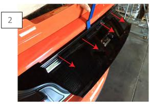
Use the panel removal tool to gently separate the factory deck lid panel from the deck lid.
