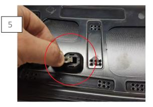
Remove the factory (4) screw clips across the bottom of the decklid panel. Transfer the clips to the MP Concepts panel
