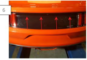
Install the MP Concepts Decklid panel to the car, and push the panel up engage the clips. Then fasten the (4) 7mm screws to bolt the decklid panel in place.
