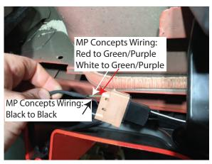
**Step 3**Connect the MP Concepts wiring to Factory wiring harness as follows.
