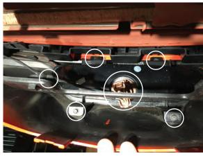
**Step 2**Pull the valance down to gain access to the (4) factory reverse light screws (7mm). Un-clip the plug on the factory light and remove the harness from the housing. Install the MP Concepts light the same way the stock light came out. Re-use the (4) factory screws.
