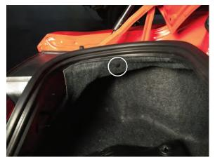
**Step 6**Using a panel removal tool or pliers, remove the plastic clip holding the trunk liner in place.
