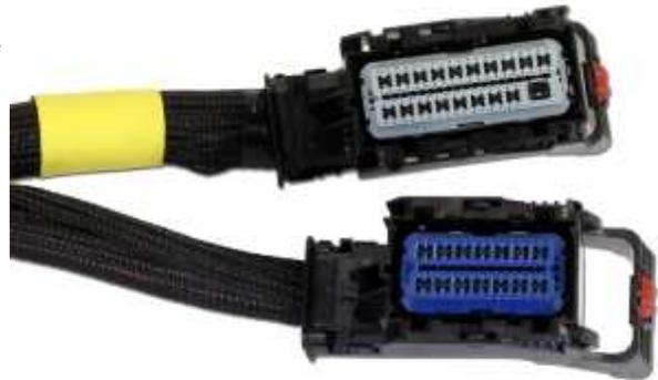
**ECU C2** - This 56-way connector should be plugged directly into the AEM Infinity ECU. This ECU is identified by the blue terminal position lock, and mates to the blue connector on the ECU.
