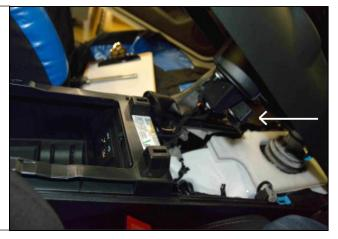
7. Remove the shift boot. There are three clips holding the boot to the reverse lock out sleeve, use a screw driver to pry one clip at a time while pulling up on the boot. Set the boot aside for reinstallation later.
