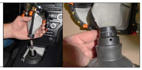
50. Install the three supplied set screws and evenly tighten the shift boot into place.
