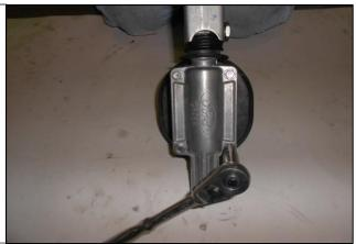
27. Remove the bottom Plate. Take care when removing the bottom plate, there is a rubber gasket that will be reused.
