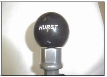
55. Check for proper operation by engaging the reverse lockout and making sure the shifter will go into reverse.
