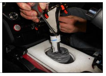
8. Once the rubber boot is removed continue by removing the plastic ring and the rubber O-ring. The plastic ring and rubber O-ring will be re-used .
