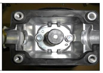
Working in reverse order from step 29 to 24, reinstall the factory shift rod and assemble the shifter housing. Re-torque all bolts to factory torque specifications apply grease to all pivot points.
