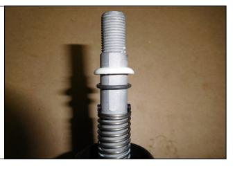
9. Remove the spring retaining roll pin and the spring. The spring will be reused.
