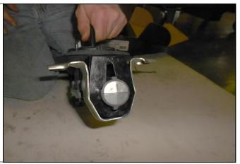
39. Working in reverse order step 21 through step 11, reinstall the shifter housing assembly, driveline, crossmember and exhaust if undone. Re-torque all bolts to factory torque specifications.
