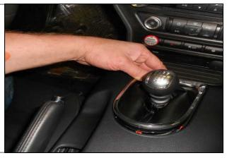
5. Remove the center console. Start by releasing the locking tabs at the rear of the console while working your way forward.
