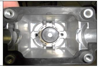
36. Reinstall the shifter retaining plate. The plate should seat flat against the bottom of the shifter housing. Torque to the factory specifications.
