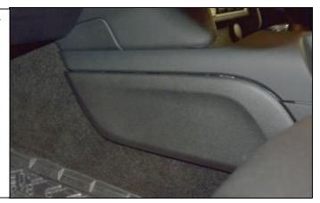
49. Install the factory shift boot onto the reverse lockout. There are three threaded holes in the upper portion of the lockout align the notches on the shift boot to the holes on the reverse lockout and push the shift boot down into place.
