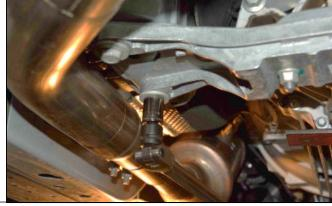
15. Remove the three (3) 15mm bolts securing the crossmember to the transmission.
