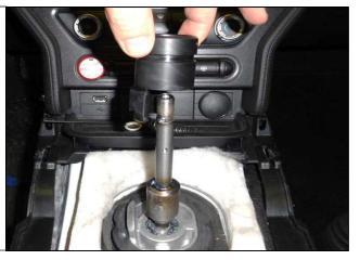
41. Align the reverse lockout block to the threaded hole on the larger portion of the Indy shifter. Use the retaining screw that was removed in step 9 to secure the reverse lockout into position.
