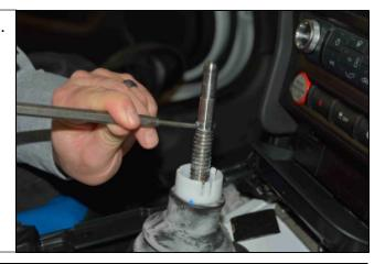
10. Remove the retaining screw and then remove the factory reverse lockout sleeve and rubber boot. The retaining screw and rubber boot will be reused.
