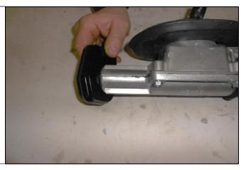
38. Insert it into the bracket clip. You will need to form the clip bracket around the new bushing to make it easier for install. The holes need to be 4.21 inches apart to be re-installed. It will be improbable that you will get it to hold at 4.21 inches apart, but try to get it close to 4.21 inches as possible. You will rely on a pair of channel locks to compress the assembly during install.
