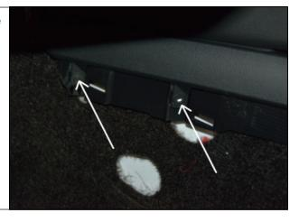
4. Unsnap the shift boot bezel from the console. Lift from the top to release the top clips and then use the pry tool to un-clip the rest.
