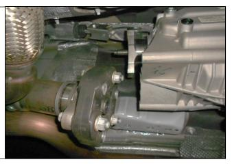
19. Remove the two (2) 10mm hex nuts that mount the rear of the shifter to the transmission tunnel.
