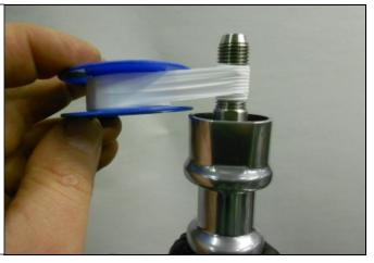
53. Apply the included LOCTITE® 271 thread lock compound to the threaded portion above the Teflon tape.
