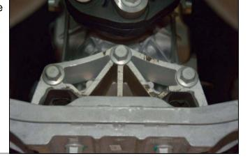
16. Remove the three (3) 18mm bolts securing the front end of the driveshaft to the transmission.
