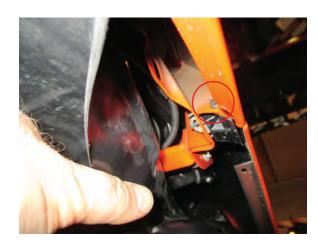
**Step 5**Fold back the fender liner so that you can access the (1) 7mm bolt that holds the bumper to the fender. Once removed, firmly pull the sides of the bumper away from the fender.
