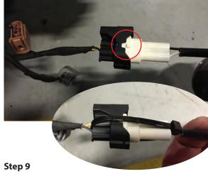
Connect the fog light to the factory fog light plug. The plugs are keyed as seen above. \*\*Note: It is recommended you zip tie the plugs together to ensure they do not come loose.
