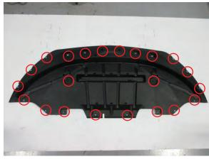
**Step 3**Support the front of the car so you can access the bumper splash shield. \*\*Note there are two versions of the splash shield. Both are attached to similar locations.
