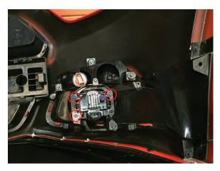
**Step 7**Using a 7mm socket, remove the (3) screws holding the factory fog light to the bumper bracket.
