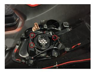
**Step 8**Install the Halo fog light using the(3) factory screws onto the factory bracket. Clean the bumper bracket and attach the halo control module using the provided double sided tape. Zip tie any excess wiring out of the way.
