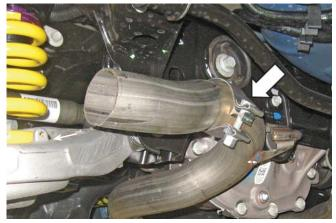
3. Insert the LoudMouth<sup>™</sup> muffler hanger into the mount at the rear of the vehicle, and then slide the new pipe over the vehicle side pipe.
