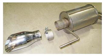
6. Check the exhaust system for proper clearance under the vehicle and also for tip alignment as shown below. If alignment is off, loosen the required band clamp, adjust, and re-torque the band clamp.
