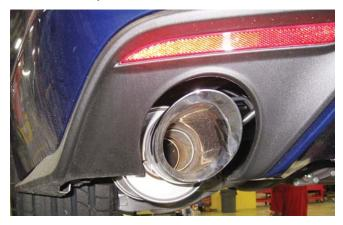
Once the desired position and alignment has been achieved, ensure all band clamps are torqued to 30 Nm.
