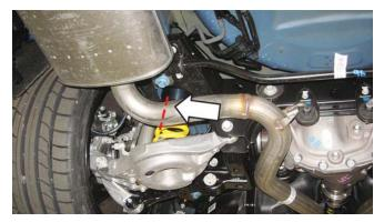
2. Cut the LH and RH exhaust pipes at the locations marked in Step 1 using a reciprocating saw with a metal blade.
