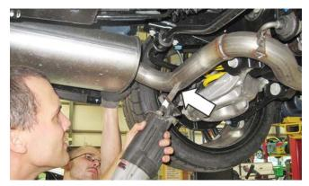
3. With the pipe cut; slide the hanger out of the rubber mount and remove the muffler assembly from the vehicle.
