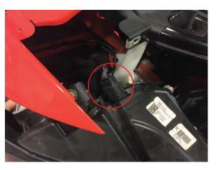
**Step 8**Once the headlight is unbolted from the vehicle unplug and remove the wiring harness from the light.
