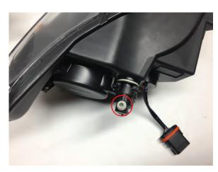
**Step 10**Using a Phillips or Allen key, use the attached adjustment screw to adjust the headlight to the factory specifications which can be found in the owners manual.
