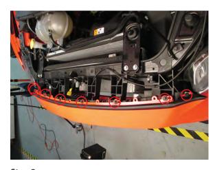
**Step 2**Remove the (6) 8mm and (2) 5.5mm bolts securing the bumper cover to the radiator support.
