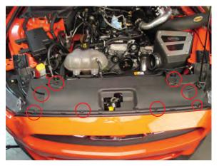
**Step 1**Remove the (8) clips securing the plastic radiator cover to the radiator support and remove it from the vehicle.
