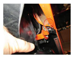
**Step 5**Fold back the fender liner so that you can access the one bolt that holds the bumper to the fender. Once removed, firmly pull the sides of the bumper away from the fender.
