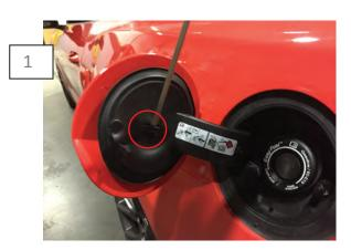
Open the factory fuel door. Using a small flat head screw driver, apply light pressure on the center clip.
