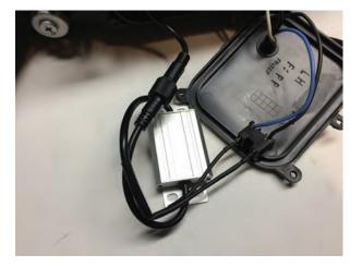
**Step 3** Connect the LED control box and plug the control box into the headlight connector. Place the control box and harness inside the headlight. Then reinstall the bulb cover.
