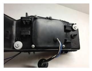
**Step 1** Remove the (4) screws securing the headlight bulb cover to the headlight, remove cover.
