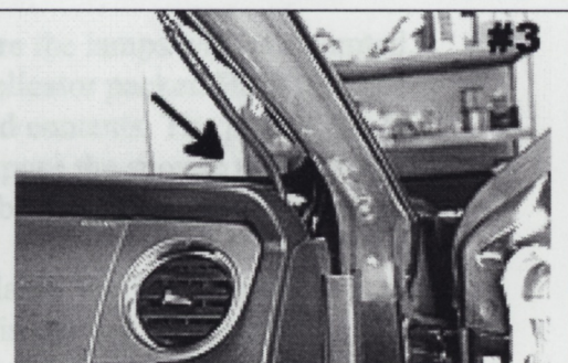
Run wiring/ lamps through gap near a-pillar to passenger side floor.
