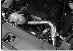
23. Re-install the intake system or stock air box. Make sure to connect the crankcase line and diverter valve return line. PF9091P intake svstem shown above.
