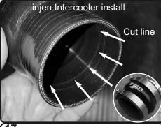
With injen Intercooler only, locate inside the hump hose for the cut indicator line. Cut back the intercooler hose at this 1" line. This will allow for the hump hose to be 2.5" x 2.5"L. Cut only with injen intecooler
