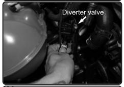
22. Re-connect the diverter valve harness.
