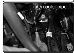
**20.** With soap water lubrication on the inside of the hump hose. This will allow for the elbow hose to slide on easier to intercooler. Tighten clamp using 8mm
