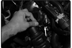
**8.** Loosen the clamp on the turbo for the hot side of the intercooler pipe using 7mm nut driver or ratchet. Loosen the clamp on the intercooler side also.
