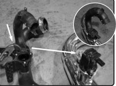
14. With pliers loosen, loosen clamp and pull back line. Carfully remove and transfer to the new injen intercooler fitting.
