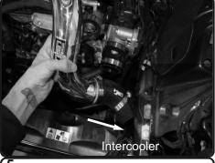
**5.** With soap water lubrication on the inside of the elbow hose, install the intercooler assembly into vehicle with clamp. This will allow for the elbow hose to slide on easier to intercooler. Do not tighten.
