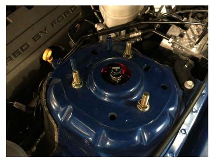
Wash the Strut Towers with soap and water. Allow the strut towers time to dry. \*\*Recommended: Wipe the Strut tower down with isopropyl alcohol to ensure the cleanest surface possible.
