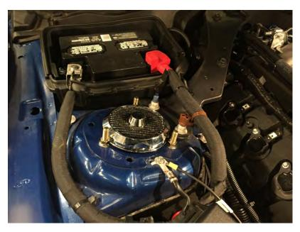
Before removing the tape backing, test fit the part. The notches align with the strut nuts/studs. Peel the tape backing and install.
