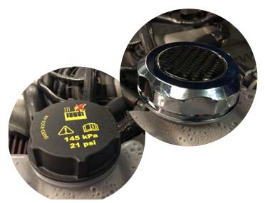
**Radiator Cap Cover:** Wash the coolant reservoir cap with soap and water. Allow the cap time to dry. \*\*Recommended: Wipe the cap down with isopropyl alcohol to ensure the cleanest surface possible. Peel the tape backing and install on the factory cap.
