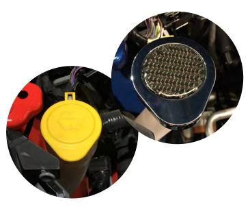
**Windshield Reservoir Cap:** Wash the windshield washer cap with soap and water. Allow the cap time to dry. \*\*Recommended: Wipe the cap down with isopropyl alcohol to ensure the cleanest surface possible. Peel the tape backing and install on the factory cap.
