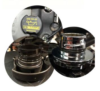
**Oil Cap Installation**: Remove the factory oil cap by turning it counter-clockwise. Transfer the oil cap o-ring to the replacement cap.
