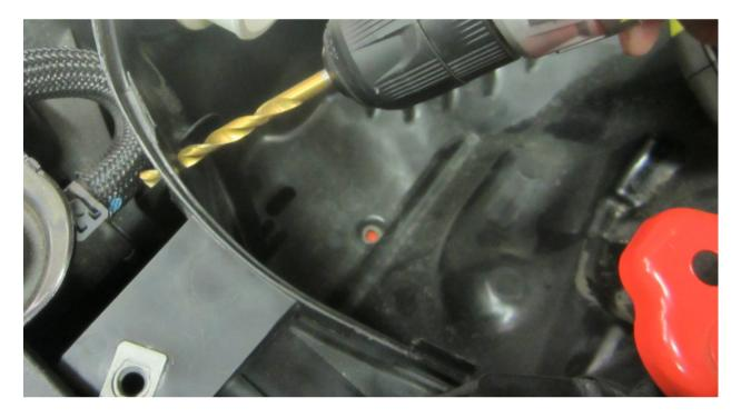
Drill hole for harness retainer.
