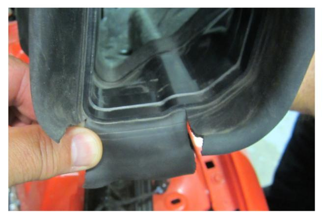
Modify air inlet by cutting rubber seal. Install inlet on air bucket
