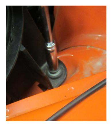
Position air bucket and install bolt. Make sure modified rubber seal on inlet is folded down by reaching your hand into the inlet. Torque bolt to 71 lb. in.
