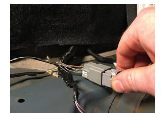
**Step 5** Install the Raxiom light. Connect the electrical connection and tighten the factory nuts.
