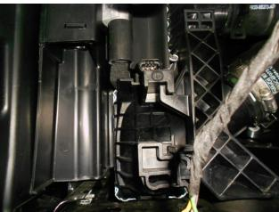
6. Connect the male connector on the Delta Boost module into the factory sensor. Connect the female connector on the Delta Boost module with the connector on the factory harness
