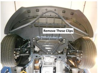
4. Carefully pry the inner fender well back to expose the driver side of the intercooler. Locate the factory boost sensor.
