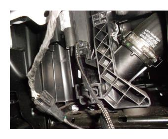
Secure the module onto a factory hole on the inner fender core support using the supplied plastic tie as shown in photo.
