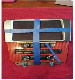
5. Flip over. Place magnets on opposite side to find the exact location. Scuff up plastic and apply super glue and place magnets. Let sit for 5-10 minutes
