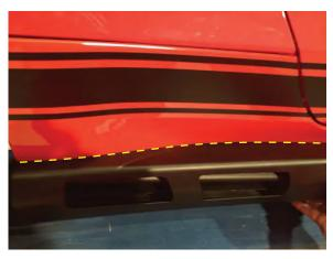
3) Once the adhesion promoter is haze, peel the backing off the 3M double sided tape and install the rocker. It is helpful to install the rocker on an angle so that the innermost edge touches the factory rocker first, then lay the rocker down. Apply firm pressure to ensure proper adhesion.
