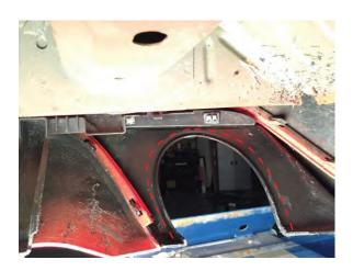
1) Clean the back side of the rear bumper around the factory exhaust cut outs of dirt and debris using soap and water. Once thoroughly dry, wipe the back side of the factory exhaust cut out with the supplied alcohol wipes to ensure a wax and grease free surface. Then apply the supplied adhesion promoter, allow the adhesion promoter to haze prior to adhering the MMD exhaust cut out deletes. Apply firm pressure to ensure proper adhesion.
