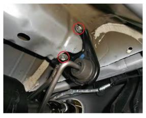
2) Place a stand under the center resonator as well as under the rear muffler assemblies. Using a 13mm wrench, loosen the two hangers just behind the rear differential from the cross member and the two hanger mounts at the rear of the vehicle from the frame.
