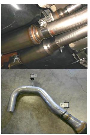
3) Place a provided clamp onto the inlet of both **815525-Z** mufflers and slide them onto the back of the 86385S Scavenger assembly. Slide them past the marks at 2.00" to allow for the installation of the tailpipe assemblies. Place a provided clamp onto the outlets of each muffler in preparation for installing the tailpipes.
