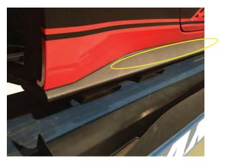
2) Clean the factory side skirt of dirt and debris using soap and water. Once thoroughly dry, wipe the top of the factory side skirt with the supplied alcohol wipes to ensure a wax and grease free surface. Then apply the supplied adhesion promoter, allow the adhesion promoter to haze prior to adhering the MMD side skirt to the vehicle.
