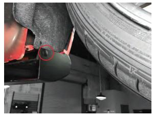
4) Remove the rear wheel to gain access to the inner wheel well. Line up the top edge of the MMD side skirt and the factory side skirt, drill a 1/4" hole through the MMD side skirt and the factory side skirt, then install the supplied push clip.
