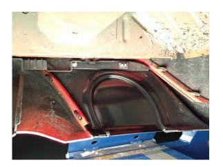
2) Peel the 3M tape backing off and install the cut out delete to the back side of the bumper.
