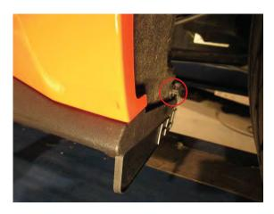
1) Remove the factory mud flap. Remove the torx head screws and push clips holding it to the vehicle.
