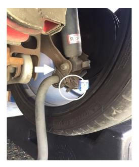
4. Once free, remove sway bar from underneath the car
