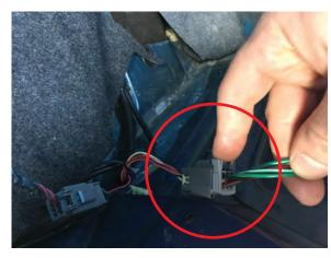
**Step 3**Unplug the factory tail light harness, and remove.
