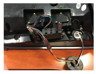
**Step 4**Connect A to B to get the lights to sequence with the turn signals. Connect A to C to bypass the sequential turn signal.
