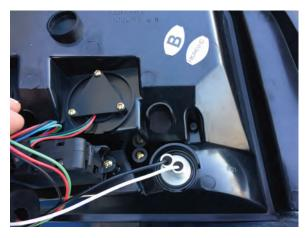
**Step 5**Transfer the factory reverse bulb into the new tail light.
