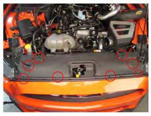
**Step 3:** Remove the 8 bolts securing the bumper cover to the rad support.
