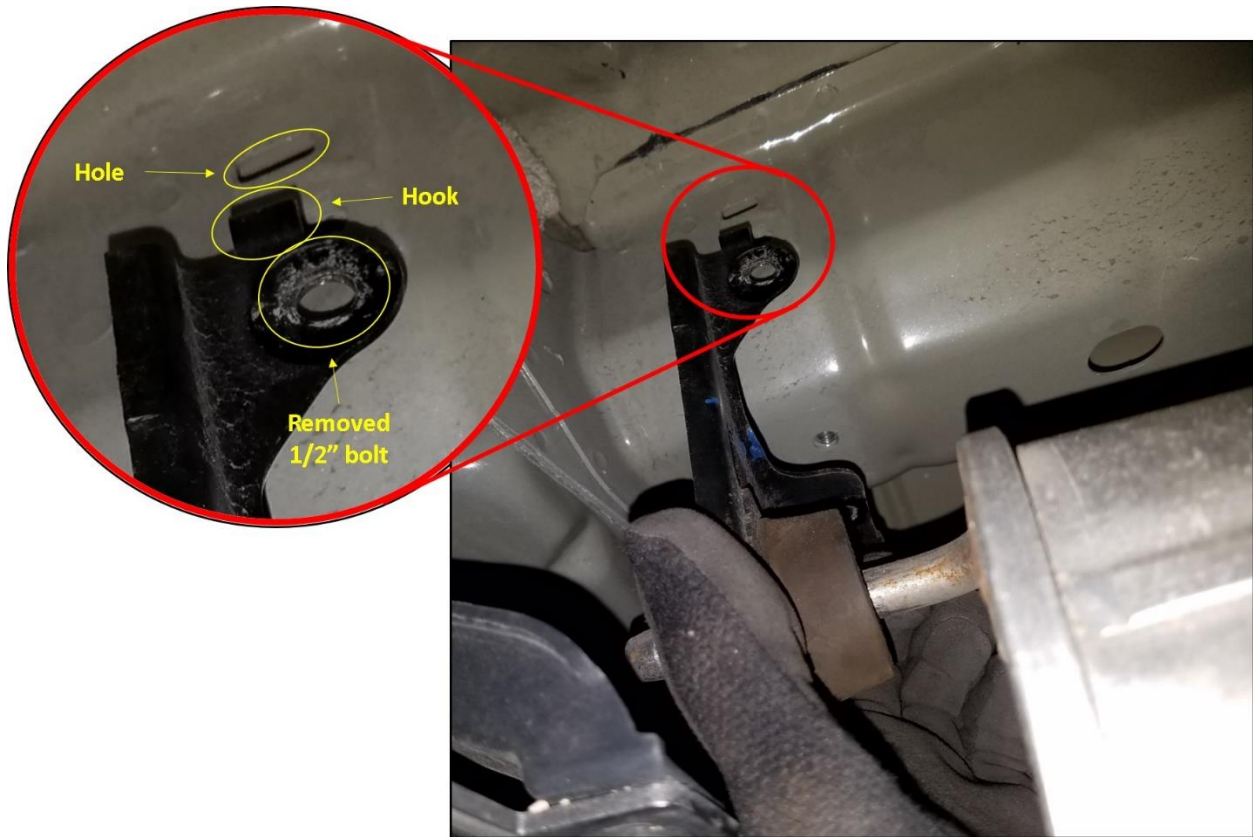
Fig. 2.4 Right and left muffler assembly bracket removal.
