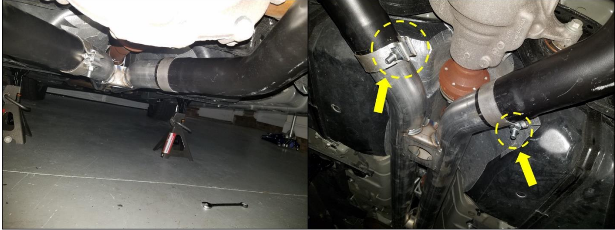
Fig. 3.7 Intermediate pipes adjustment.
