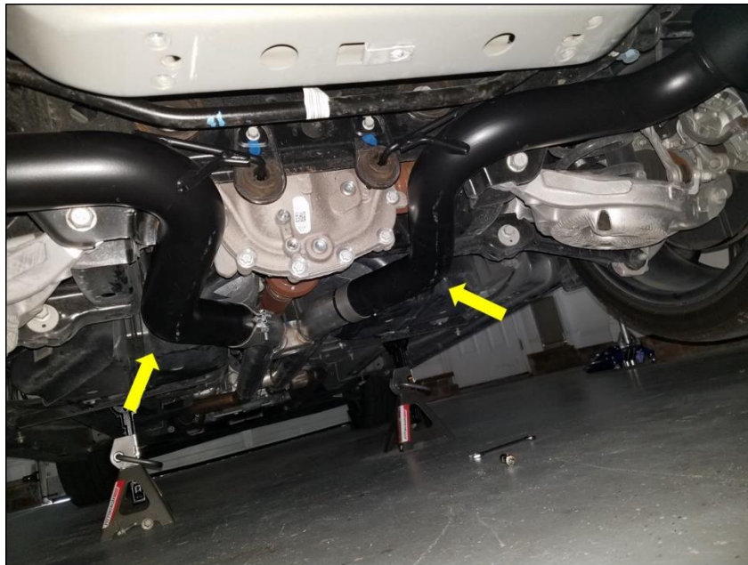
Fig 3.6 Ensure intermediate pipes are adjusted up high enough.
