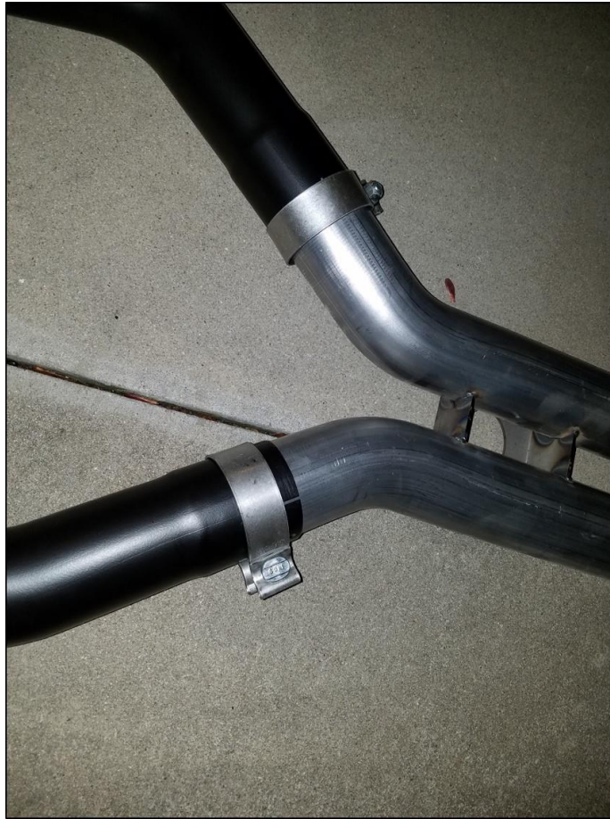
Fig. 3.2 Intermediate pipes to H pipe connection.
