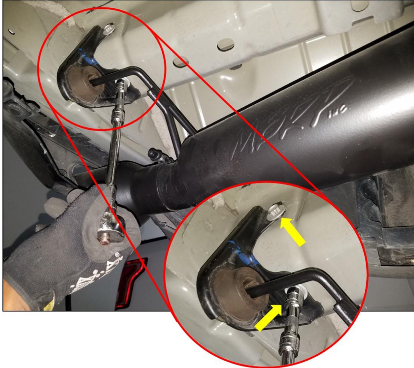
Fig. 3.5 Hang exhaust assembly brackets.
