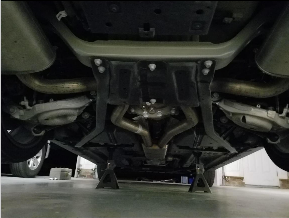
Fig. 2.1 Frame Brace removal (If applicable).
