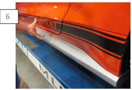
Angle the rocker to ensure the panel is placed as far back as possible. Press the rocker flat, and apply firm pressure to the length of the panel.
