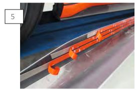
Remove the double side tape backing.
