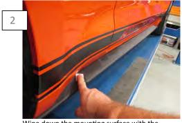
Wipe down the mounting surface with the supplied alcohol wipe, and then adhesion promoter.
