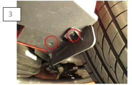
Remove two torx screws and plastic retaining clip holding the plastic splash shield. Remove shield
