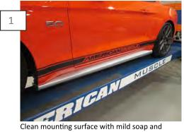
Clean mounting surface with mild soap and water allow plenty of time for the panel to dry thoroughly. Test fit the rocker to ensure you have them on the proper sided. \*\*Note: A clean surface is essential for proper adhesion.
