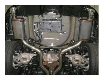
**Step 4.** Finish the initial installation by fitting the Muffler Assemblies onto the Extension pipes using the supplied 3.00" clamps and inserting the hangers into the rubber insulators.
