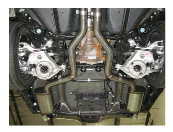
**Step 3.** Next attach the Extension Pipe Assemblies to the X-Pipe using the supplied 3.00" clamps and fitting the hangers into the rubber insualtors.
