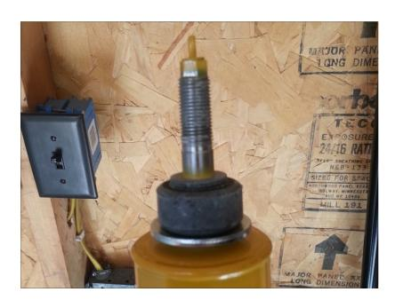
2) Remove top nut and bushing from stock shocks using adjustable wrench (may need locking pliers on the threads for the final few turns) and 9/16 inch wrench as pictured.
