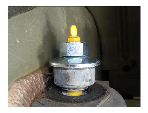
8) Tighten the nut with ¾ wrench until the bushing bows out, do not flatten the bushing. It may be necessary to hold the top of the strut with the 9mm wrench to keep it from turning. Install the top nut as a lock nut using the ¾ wrench to hold the bottom nut and the socket to tighten the top nut together.
