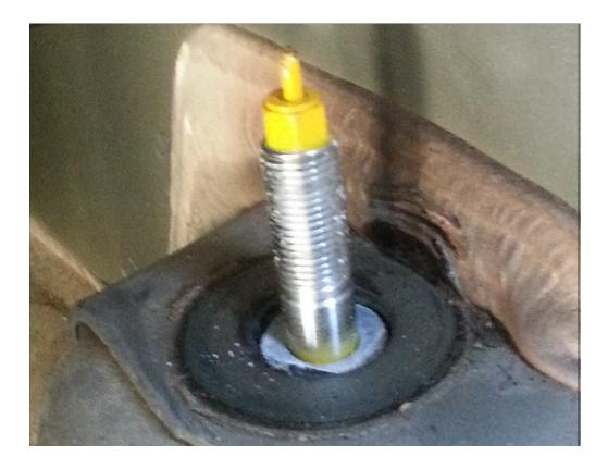
7) Install a bushing, washer, and nut on the top of the shock. Press the top bushing to align the raised section is in the hole like the bottom bushing.
