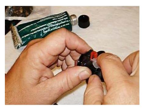
7. If replacing spark plug, be sure the plug is properly gapped and threads coated with anti-seize.
