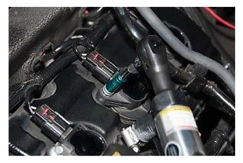
3. Slide red locking mechanism back on coil/plug wire and release from coil.
