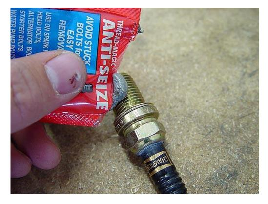
8. Using the 5/8 deep socket, replace the spark plug.
