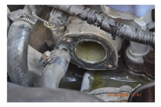
6. Take off old gasket & clean areas were the gasket was removed. I used a razor blade scraper & finished with 60 grit sandpaper
