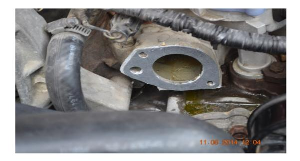
11.Put washers on the screws and start to thread by hand (either hole) Once both are started begin to tighten all the way. (6mm hex key socket I think 12.After they are tight grab the NEW Intake piece. Start to thread by hand & finish with a 7/8 box end wrench.
