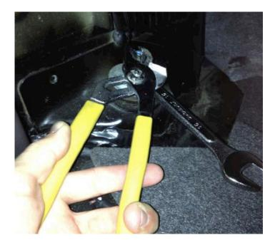
4. Once the top bolt of the shock is removed, remove the 15mm bolt at the bottom of the shock.
