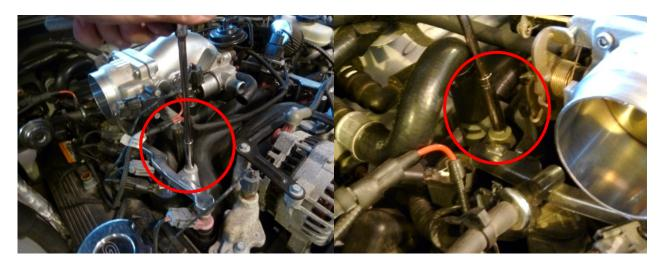
6. Get your paper towels ready for the next step. There will be some fuel left in the rails even after the engine stalls out and this fuel will be under pressure. Carefully lift the fuel rail and wiggle out the first injector, which one you do first is up to you. I did the passenger side front because it is the easiest to reach and easiest to catch remaining fuel after the injector is pulled out of the rail.
