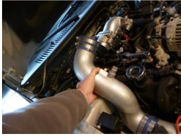
4. After removing your intake and other tubing you may have, disconnect the electrical connections to the fuel injectors.
