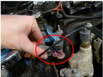
5. Using your 8mm deep socket, remove the bolts/studs holding the fuel rails to the intake manifold. There will be (2) for each side, (4) in total.
