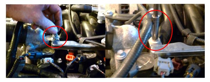
12. Reconnect the electrical connections to the new injectors and other connections that you may have had to remove from the fuel rails.
