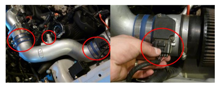
14. Reconnect the electrical connection that you had severed to shut down the fuel pump (fuel pump reset switch in the trunk for this install).
