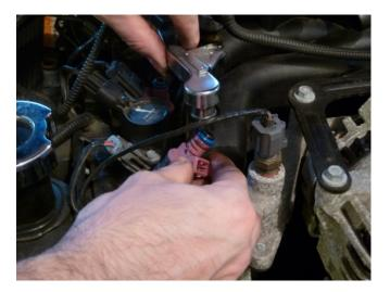
7. Carefully remove all (8) injectors and catch any fuel with paper towels. Next, I used a vacuum to suck out any dust that may have been on the injector seats.
