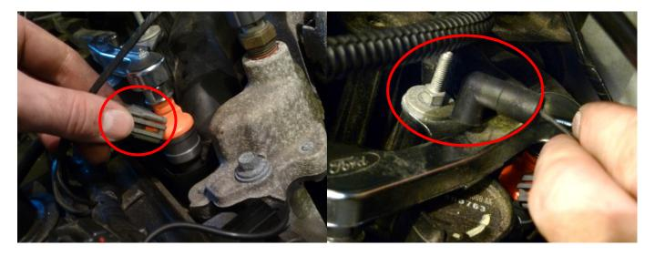
13. Reinstall your air intake and corresponding hoses, hardware and electrical connections.
