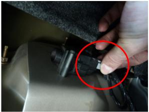
15. Next, turn your key to the ON position; do not START. This will prime and re-pressurize the fuel lines. Now that the rails have pressure, you can check to see if there are leaks. The fuel pressure should be about 45psi; if you have a leak you will know. Check each injector for fuel spraying out; run your hand around each one to see if you feel anything.
