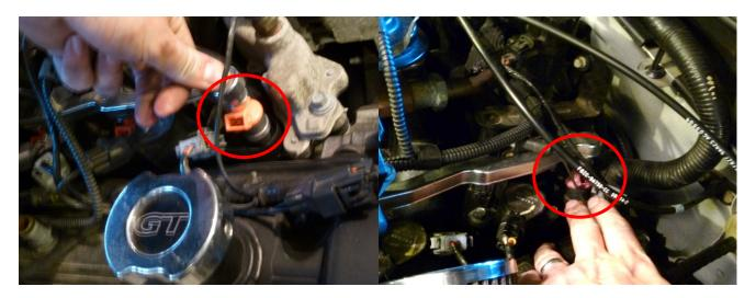
11. Replace the bolts for the fuel rails and tighten them down, alternate tightening between the front and rear bolt. Remember, the bolts are going into a plastic manifold so don't over-tighten them. Repeat on the other side.
