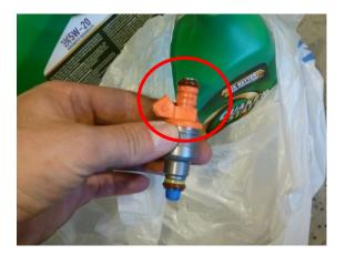
9. One at a time, place your new injector into the manifold injector seats. **NOTE:** Do not push down on them yet; just place them into where they sit in the manifold. You want the electrical connection facing outward (toward you) so you can connect it later.
