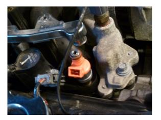
10. Gently line up the fuel rail on top of each set of 4, doing one side at a time. Make sure the tops of the injectors are lined up with the ports on the rails and the bottoms are still in the manifold seats. Very gently push down on the fuel rail on each end and then in the middle to secure the rail to the injectors. You will feel them "clip" in. Don't push too hard; they will fully seat when you bolt down the rails. Repeat this on both sides.
