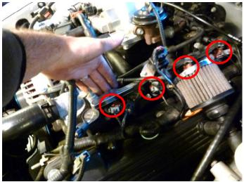
16. Start your car and recheck your injectors for leaks, then clear any codes that you may have. I used my SCT hand held tuner; if you don't have one, a local auto parts store will typically clear a code for you. Using larger injectors may require a custom/dyno tune or at least a recalibration of your computer's fuel parameters. Check with your local dyno shop.
