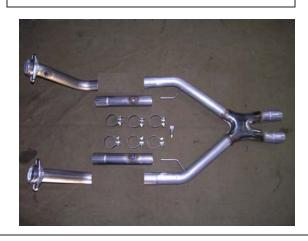
Note: anti-seize should be applied to all fastener threads and pipe slip joints
