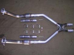
Note: anti-seize should be applied to all fastener threads and pipe slip joints
