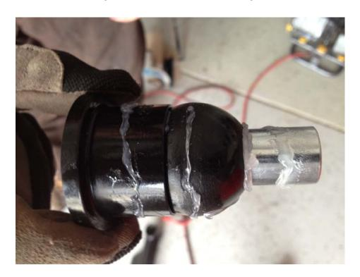
D. Using a soft hammer (plastic or wood), drive the ball and bushing into the control arm from the opposite side.
