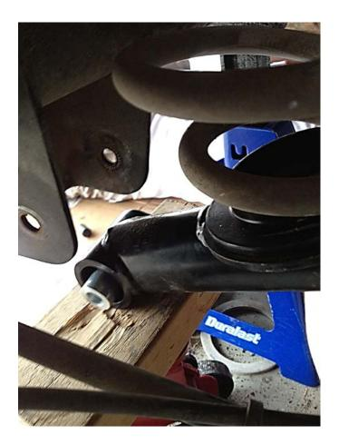
9. Remove the front control arm bolt at the body. This can be accomplished with a 18mm deep well socket on the side closest to driveshaft and a shallow well socket on the opposite side.
