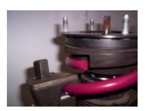
7. Once the spring is compressed, remove the 21mm nut on the top of the strut. You may need to hold the strut shaft with a 10 mm wrench to prevent it from spinning. Once the nut is removed, remove the upper strut mount. We do NOT recommend using impact guns on struts or shocks.
