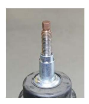
10. Place the camber plate assembly with the spring seat over the strut shaft like shown. Strut not shown for clarity. NOTE: OUR NEW DESIGN DOES NOT HAVE THE SPRING LOCATOR AS THE SPRING IS LOCATED OFF THE STRUT.
