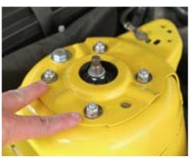
18. Install the supplied M10 x 20mm bolt with 10MM support washer into the caster slot in the factory tower. You can now snug all 5 mounting bolts and nuts.
