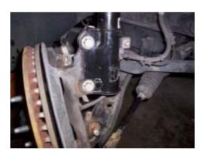
2. Remove the 18mm nut on the strut for the sway bar end link. Remove the end link from the strut by pushing it through the hole. Do Not Use Impact Gun
