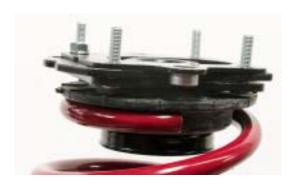
11. Place the small spacer that measures .465" total length over the strut shaft. Spring not shown.
