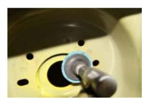
15. The camber plate has a offset bearing design which allows you to install them in a street setting or a race setting. To install in the street setting which will allow you to more positive camber for lowered cars simply install with the notch toward the inside of the car (engine side) and the race setting you will install the notch toward the fender (outside) of the car.
