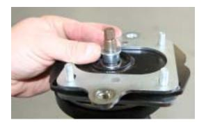
12. Re-Install the strut nut and torque to factory specifications. Spring not shown. (Do Not Use Impact Guns).
