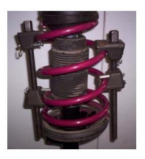
6. The spring is compressed enough when the spring has no pressure on the upper mounting plate, as shown to the right.
