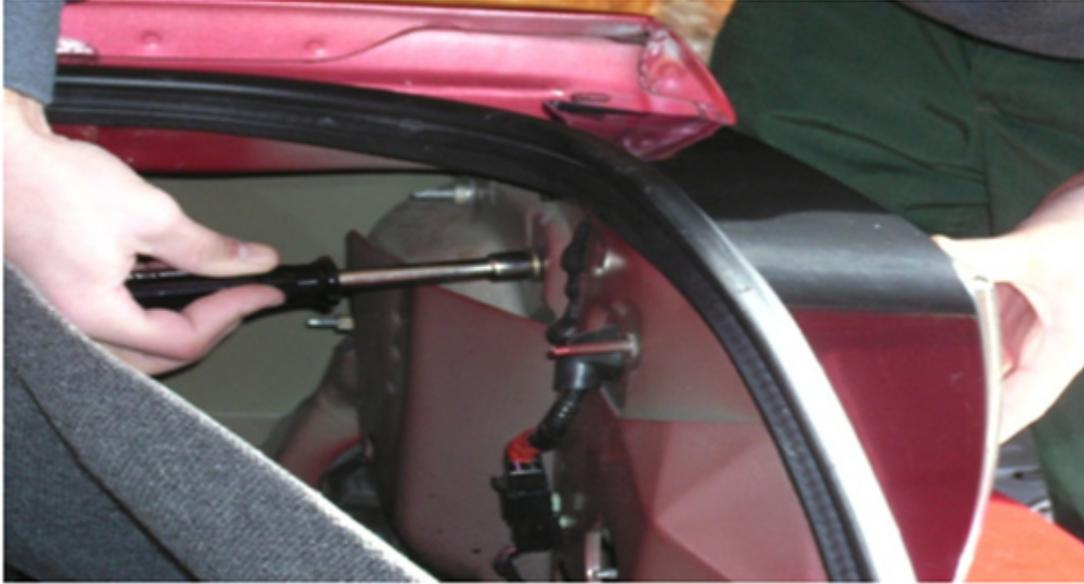
2. Drape a towel or shop rag over the bumper to avoid scratching either the bumper or the stock tail light assembly. Once the nuts have been removed, slide the tail light assembly out and place it on the towel on the bumper of the car.
