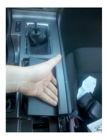
D. There will be some wires attached for traction control, flashers and the trunk. There is a small tab on the back end of the black connector, as shown by the arrow in the picture below. It is on the inner side towards the shifter. Push the tab in and pull the connector out. The gray piece will stay in the trim; only pull on the back of the black connector as shown.
