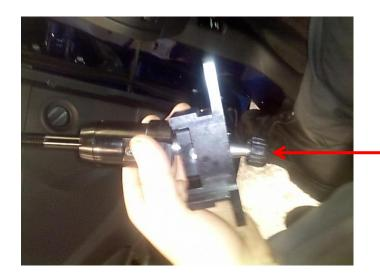
G. Place the new shifter in and make sure it sits flush with the linkage. Once it is in, take the (4) bolts and tighten them in a cross pattern; the order to tighten is numbered below.
