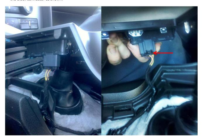
E. Remove the trim/cup holder and set it aside on the passenger seat. The picture below is a view of what is underneath the trim.
