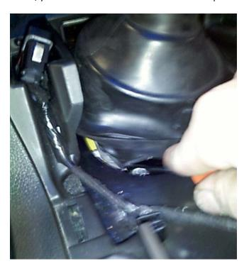
D. Once the boot is seated on the shifter, you will have to slide the edges of the boot into place around the body. Pull the top of the boot down over the shifter as shown in the picture below. It's a good idea to tuck the boot into the floor-pan for a proper seal.
