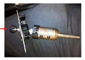
F. Once the black piece is removed, coat the ball of the new shifter with some of the white lithium grease and slide the black piece onto the Barton shifter.
