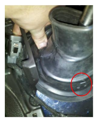
C. Pull the bottom of the boot down and set one side over the lip as shown below. This is where the mini hook tool comes in handy. Insert the mini hook under the boot and use it to pull it over the lip and it should slide in place. If you do not get the mini hook, you will need to maneuver the boot into place.
