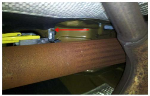
D. Pull the linkage off of the studs and let it hang freely. Go back inside the car and remove the (4) 10mm bolts from the stock shifter, as shown in the image below.
