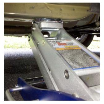
B. Secure the car on the back of the sub-frame with a jack stand. Lower the vehicle slowly, making sure it seats properly. Lift the jack back up to the vehicle as an added safety precaution in case the jack stand fails; the jack will support the vehicle for you to get out.
