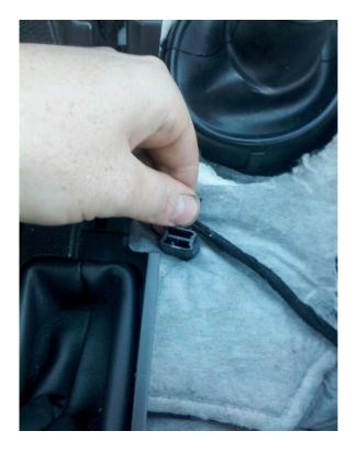
G. Next, remove the small plastic pin that holds the insulation down and set it aside. You should be able to unscrew this with your hand. If not, you can also pull up on it or use a Torx bit to remove it.
