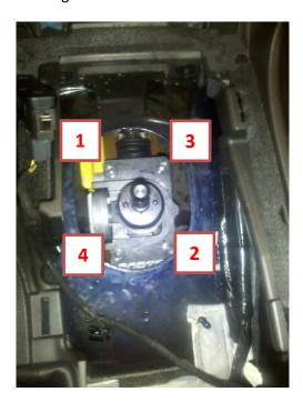
H. Go back under the car and bolt the shift linkage back up using either the stock bracket or upgrade to the Barton Shifter bracket, recommended for smoother, faster shifting. Once it is bolted back up and tight, you may lift the car, remove the jack stand and lower the car back down.
