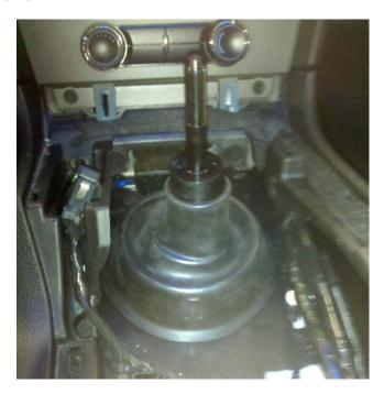
E. Reinstall the insulation, insert the pin and push the wire holder over the dowel. Insert the trim and cup holder piece. Reattach the wire connector to the traction control button. Slide the trim forward to get the tabs into the holes and lower the trim into place.
