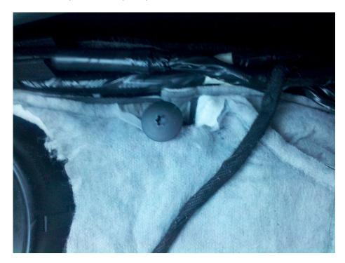
H. Lift out the insulation material and remove the rubber dust boot from the shifter by pulling up on it. Grab the boot in the spots indicated below.
