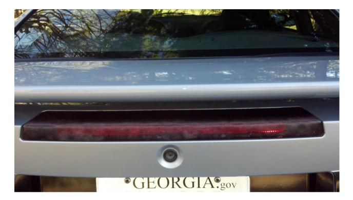
You can remove the brake light by using your 10 mm socket wrench and remove the two bolts behind the brake light, in the trunk. (I only showed one, the other one is parallel to it). There should be one black clip that connects the actual brake lights, just unclip it and remove the third brake light.
