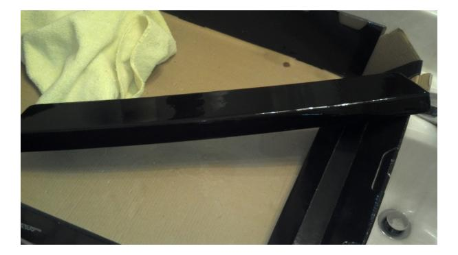
10. If you end up having a water bubble you can take a needle and poke the bubble, creating a tiny hole.You should see some water seep out. The tiny hole will heal with the sun exposure and in some time go away.
