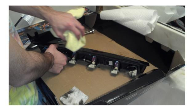
6. HEAT. Grab your hair dryer and begin the heat the tint film. DON'T NOT OVERHEAT THE FILM. BE CAREFUL. You want to heat the film along the edges of the brake light and press the excess film that hangs over the brake light around the brake light. It'll take some time to make sure the film is pressed and stuck, but really worth the effort. After that continue heat the rest of the brake light to make sure its pasted on.
